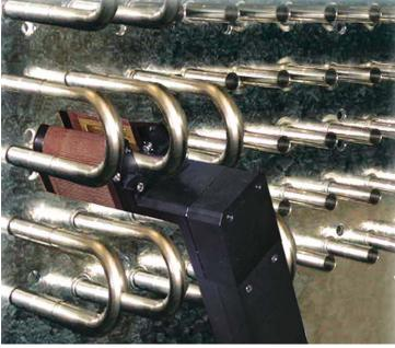
case scenario (fault in the middle of the bundle) due to the accessibility factor. With the HX head, only the affected elbow would have to be replaced. This designbased advantage also makes the Orbitalum system the ideal tool for unbeatably cost-effective repairs. The head is only 1.5 kilograms in weight. In contrast to open tongs with a cumbersome hose assembly, all connections for power, gas and cooling water are permanently integrated in the HX.
