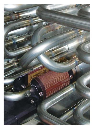
millimeters is sufficient for the HX 16 from Orbitalum for extremely easy positioning and clamping, thanks to its outer diameter of only 60 millimeters.
