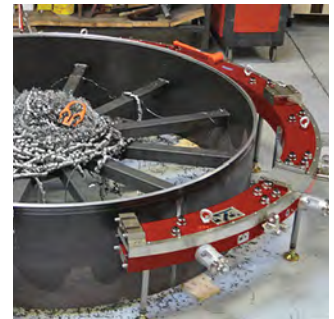
Four standard LDSF sizes cover 60in-120in (DN1500-3000)
