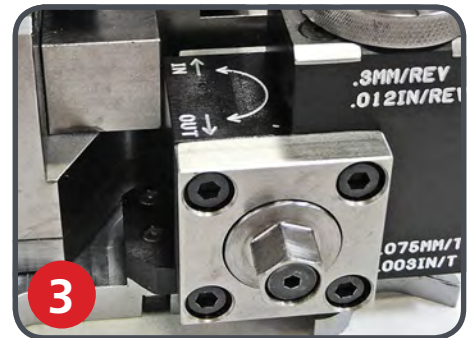
Rapid advance and retract feature speeds positioning of tooling
