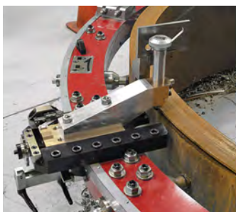
Cantilever template head loaded into parting slide base
