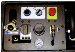
Ergonomic fingertip control with safety stop button
