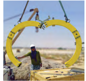
Splits open for quick, easy mounting to pipe
