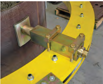
Clamping Legs speed setup and handle multiple pipe diameters
