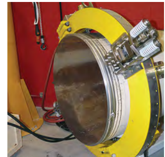
Simultaneously cuts and bevels out-of-round pipe
