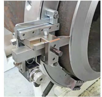
Newly designed slides with rapid retract feature
