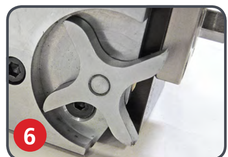
All new no-time starwheel works with newly designed trip to prevent crashing
