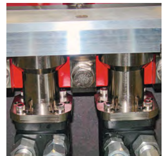
LDSF standard dual hydraulic drive motors & dual pinion housings
