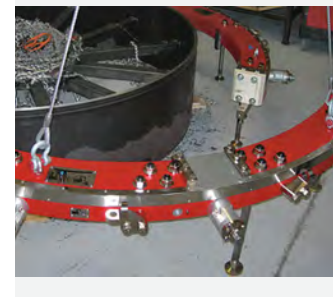
LDSF splits into quadrants for setup, transport and storage
