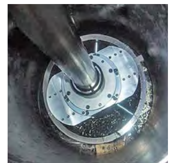
Internal cutting module lowered to cutting depth
