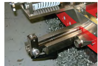
All new trip design features a breakaway mount to prevent frame damage
