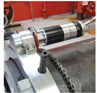
New more powerful straight shaft axially mounted air motor
