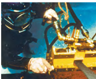
Model HE Hydraulic Trav-L-Cutter suitable for full immersion
