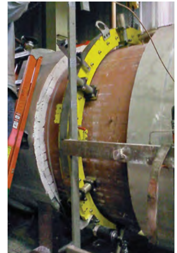
HDSF mounts to pipe exterior for precision weld preparation
