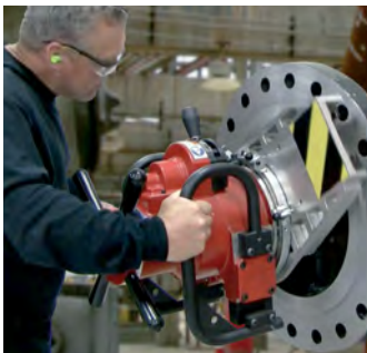
Faces flanges up to 24in (609.6mm)
