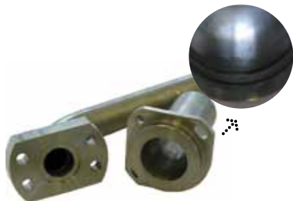
Example of internal seam weld.
