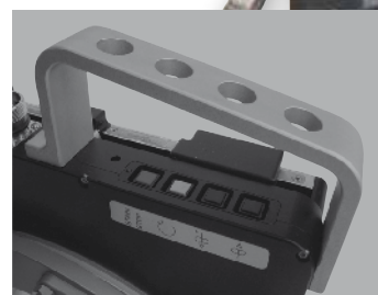
Built-in remote control panel.
