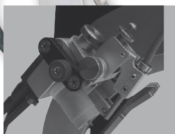
The TIG torch is mounted on a precision slide to give precise, fine control of the electrode during welding.
