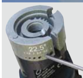
Grinding electrodes: 4 different angles and 6 different electrode sizes
