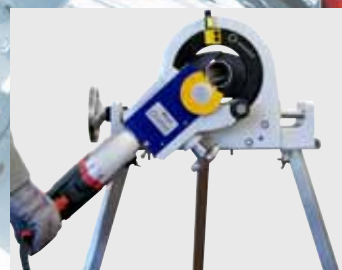
Cutting thin-walled stainless-steel tubes and elbows
